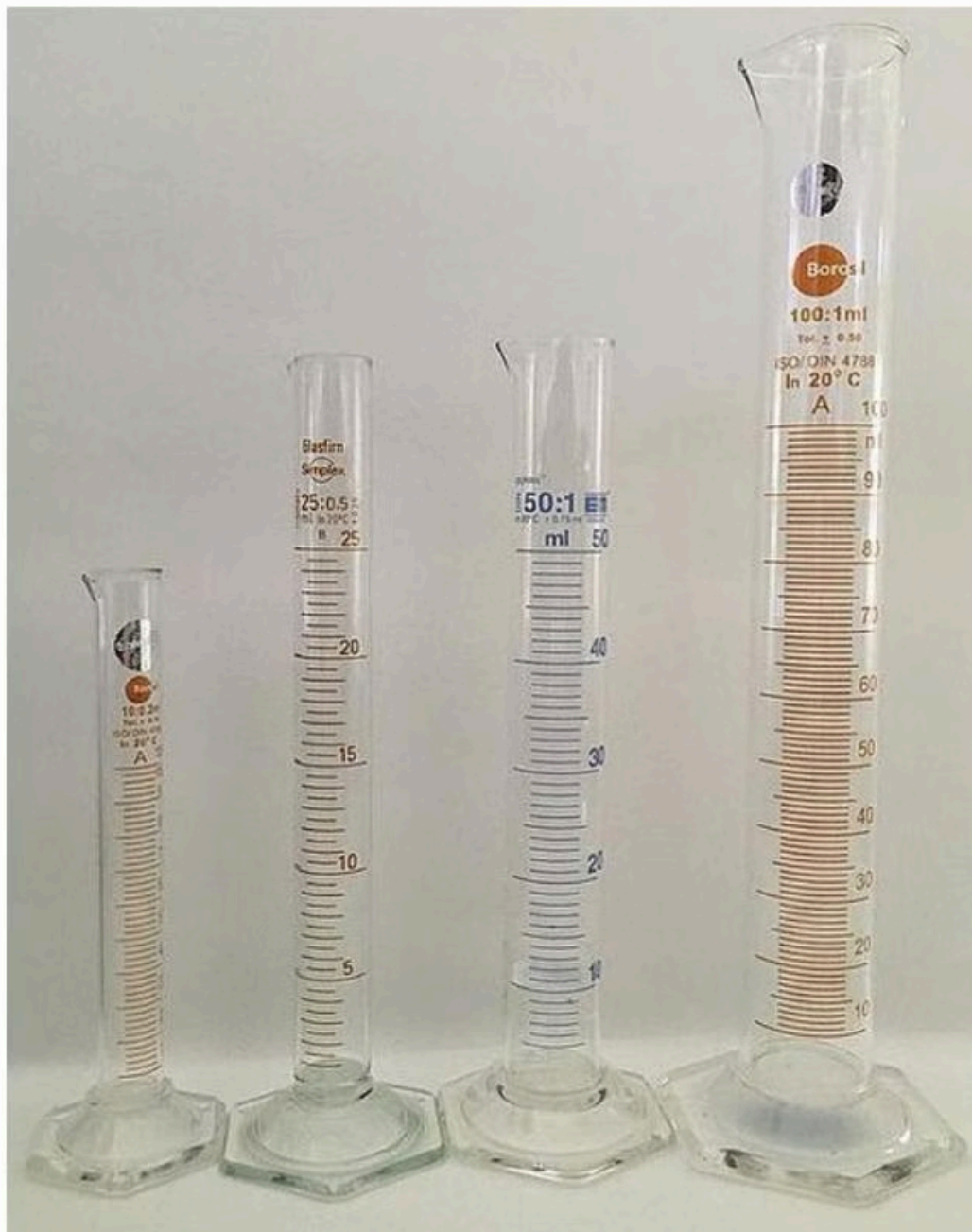
Fig. 1: Measuring cylinders used to measure volume accurately.
